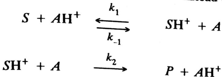
Applying steady state approximation for  $[SH^+]$ , as before, we have
